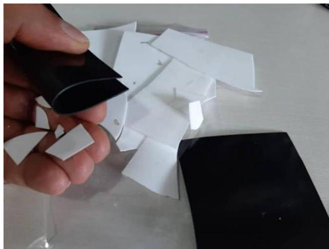
Figure 3. PP samples after 2000h of UV exposure: white pieces are PP sheets without carbon black and black sheets are PP containing carbon black.
