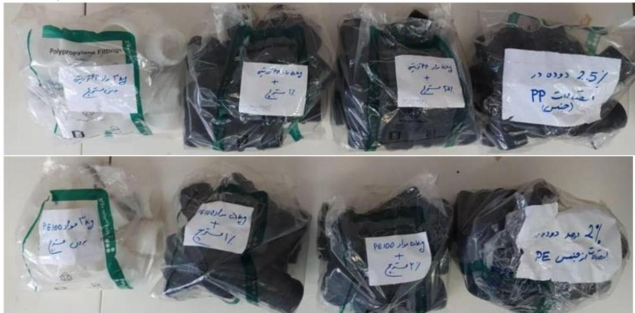
Figure 1. Injection molded HDPE and PP fittings with and without carbon black
