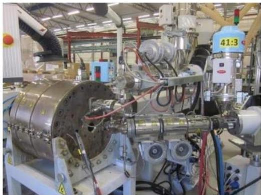
Pipe in pipe production is a further application of cross heads – In this case the production of a 3 layer (PE/Adhesive/EVOH) protection pipe over a 4 layer PE pipe for fuel transportation on petrol stations
