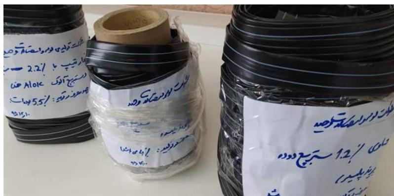
Figure 1. Irrigation tapes containing 1.2, 1.5 and 2 wt% carbon black
