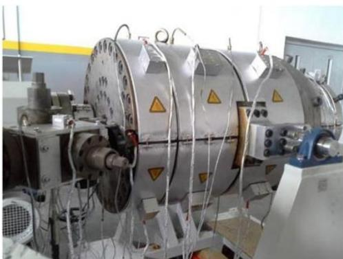
The features for multilayer heads is same – attached also a photo of a PO 3 450 up to 630 mm. The head is designed to produce 3 layer PE or PP-R pipe from 75 to 630 mm. The heads was fundamental designed by Conextru and final engineered and manufactured by Mikrosan under supervision of Conextru GmbH. The head is design for a 2 extruder version according customer requirements and is in operation in Serbia. More common is to work with 3 extruders.
