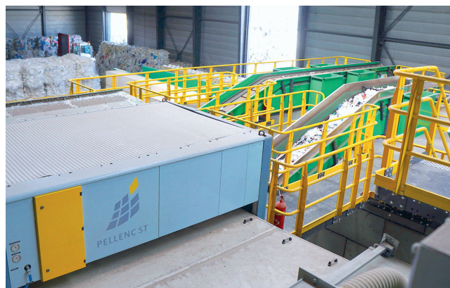
Image 3: The film bales are dissolved at DALY Plastics. They then go through a sorting process that eliminates foreign material and separates the films into color classes or material quality. This is used to produce unmixed bales, which are processed into granules in the recycle plant
