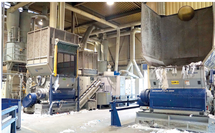
Image 4: The un-mixed film-bales are processed into film flakes in granulators, which are then fed batch wise to MAS DRD dry cleaners where granular soiling and moisture are removed
