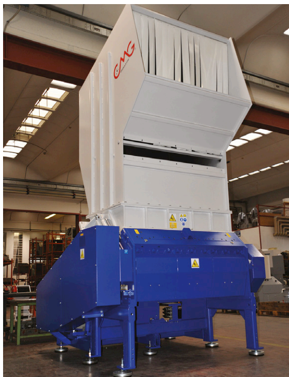
Right: CMG's EV616 granulator is part of its Evoluzione series
