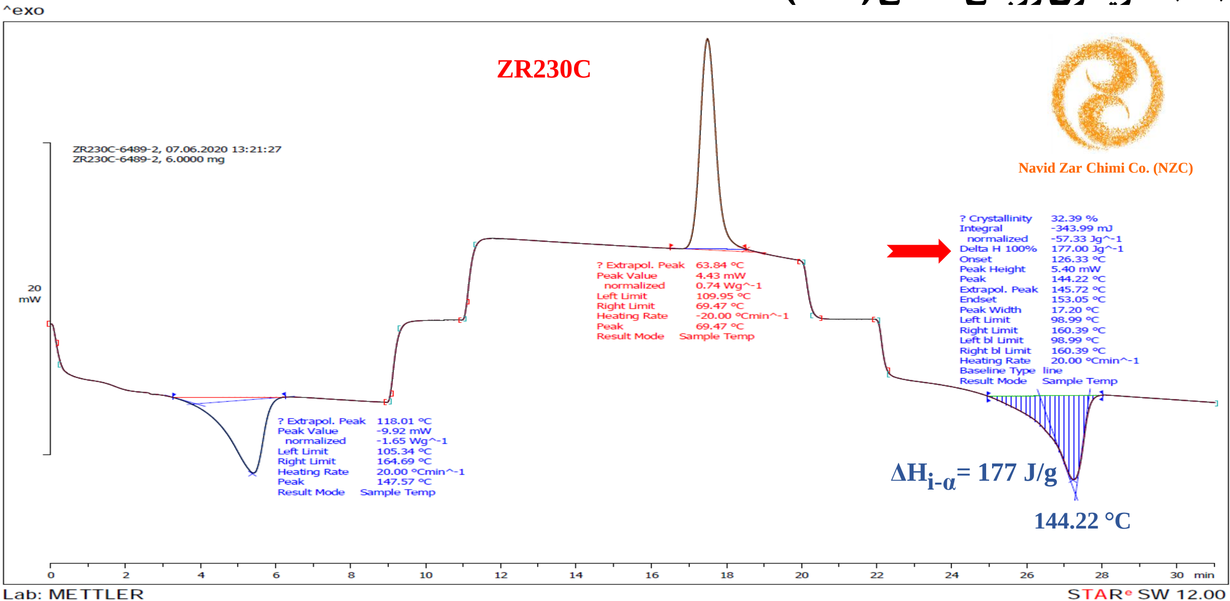
Fig. 12: Heat-cool-heat DSC scans for beta-nucleated Homo- PP sheet.
