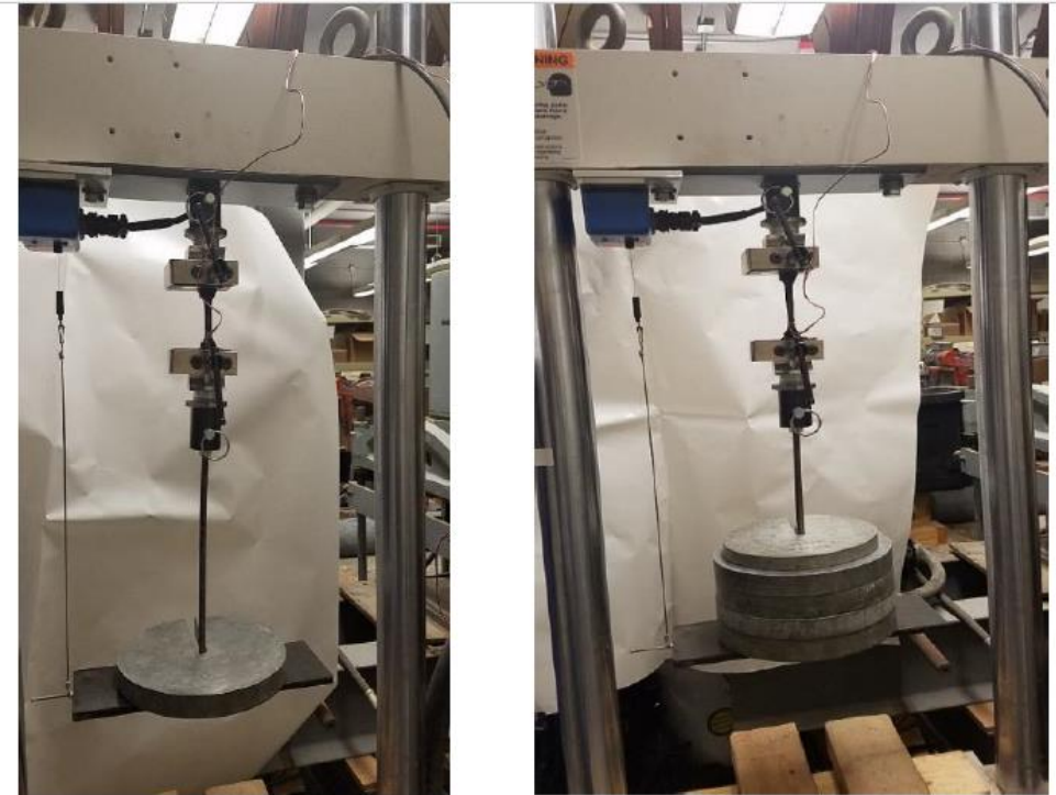
Loading the HDPE Pipe Specimens Using SSM Load Frame
