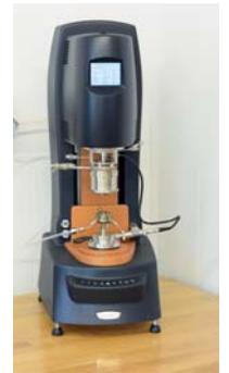
*TA Instruments Discovery HR-2 Hybrid Rotational Rheometer*
