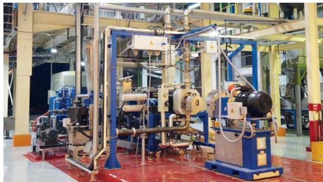
New polypropylene pelletizing line in Indonesia, with Useon's SAT-X 175 co-rotating twin-screw extruder; skid-mounted BKG® underwater pelletizer is in foreground
