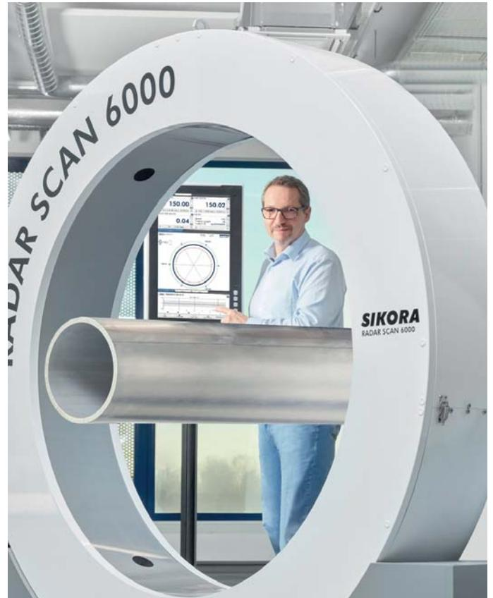
the processor system ECOCONTROL 6000. Furthermore, extensive trend and statistical functions as well as comprehensive data logging are available. The RADAR SCAN 6000 contributes to the highest product quality, process optimization and cost saving during tube manufacturing.
