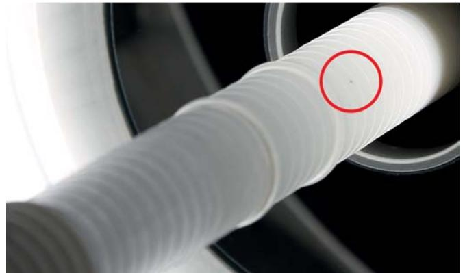
With the new inline gauge ProfilControl 7 S Corrugated Tube developed by PIXARGUS it is now possible to inspect the complete wavy structure of corrugated tubing gaplessly.
