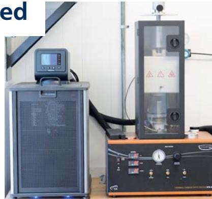
*TA Instruments DTC-300 Thermal Conductivity Meter*
