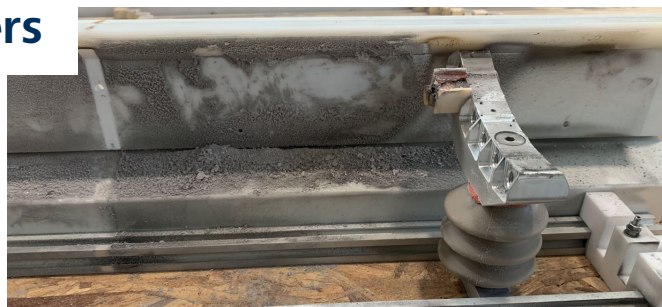
A visual reminder of the importance of keeping electrodes clean if they are to function correctly
