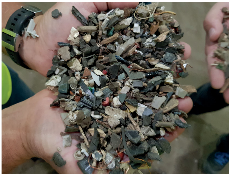
The input material contains valuable metals but also glass and minerals
