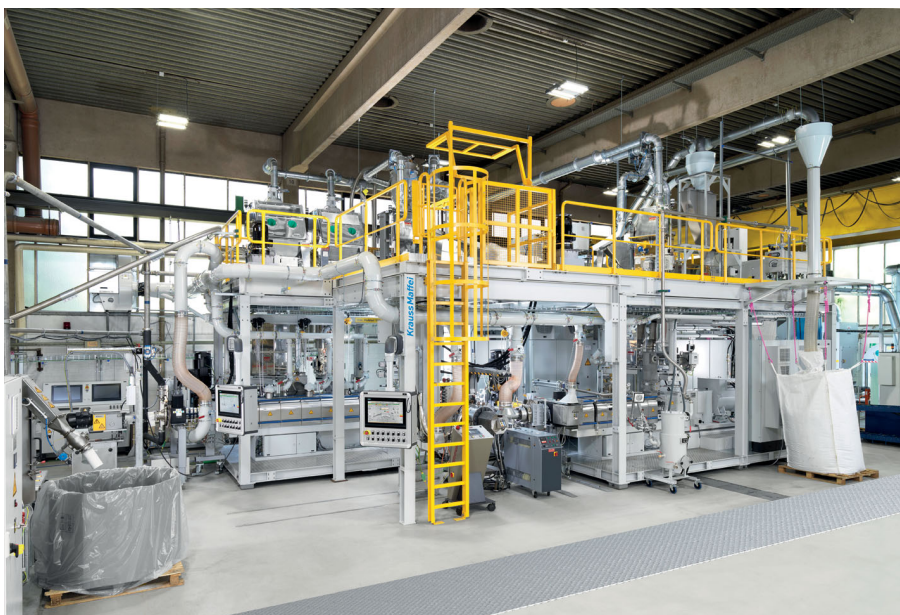
KraussMaffei has invested in a new Edelweiss compounding, recompounding line, which is now ready for customer trials
