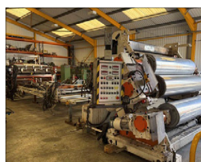
1850mm Davis Standard Sheet Downstream with 450mm diameter rolls inclined
